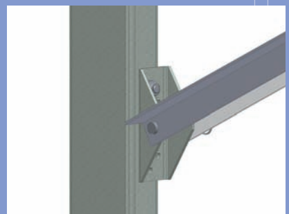
Supporting profile fixed to pile with U-bracket
